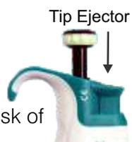
To eject the tip, point the pipette at suitable waste receptacle and press the ejector with your thumb.
