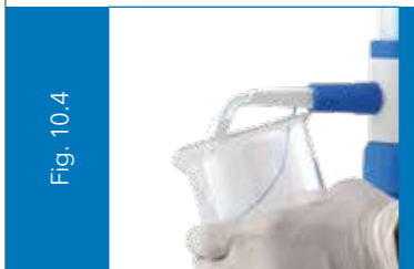
Hold the discharge tube orifice against the inner wall of the appropriate receiving vessel. (Fig. 10.4)
