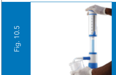
Gently lift the piston until the upper end. Press the piston downwards slowly and steadily with minimal force until the lower end. (Fig. 10.5)
