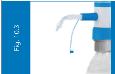
Remove cap from the discharge tube. (Fig. 10.3)
