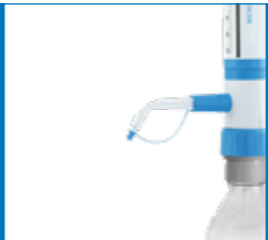
Reattach the cap to the discharge tube. (Fig. 10.6)
