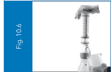
Gently lift the piston until the upper end. Press the piston downwards slowly and steadily with minimal force until the lower end. (Fig. 10.6)
